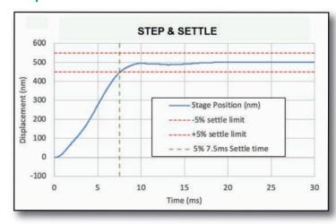
Settling time of the NanoScan OP400 stage with NPC-D-6110 controller with 150g load.
