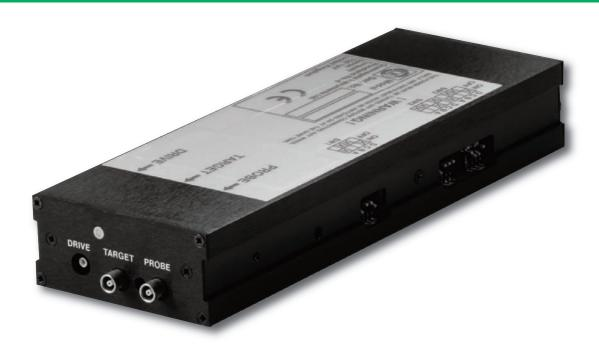
The NPS2101 and the NPS2100-20 are NanoSensor, high voltage amplifier and control electronics combined as a single channel standalone module, powered by an external ±15V, 130V and -30V DC supplies.
