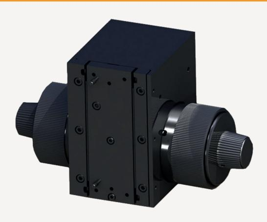
The FB201 from Prior Scientific is a manual focus block, ideal for OEM applications requiring manual, fine focus adjustments. Rack and pinion mount allows smooth, precise focussing over 29 mm of travel. A large coarse focus mechanism incorporates a slip clutch and focus adjustment. Fine focus adjustment control is graduated in two micron divisions throughout the fine focus range. The focus block can be easily adapted to various mounting configurations.
