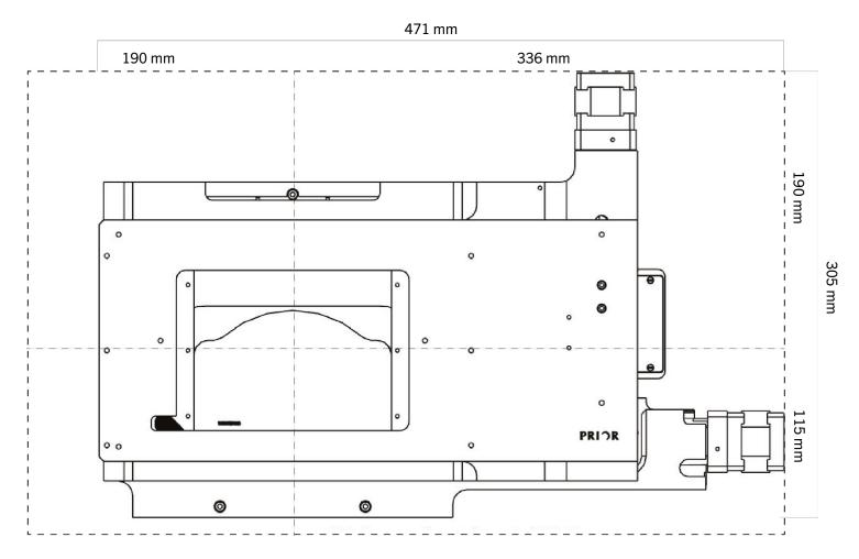
\*Outer dotted line shows the maximum footprint of the stage when at the limits of travel.
