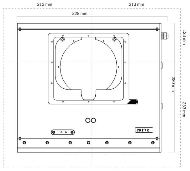
\*Outer dotted line shows the maximum footprint of the stage when at the limits of travel.
